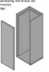
500 mm base element for condensate drip container with cutout for cleaning hatch
