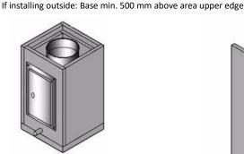
500 mm base element with cutout for cleaning hatch and side condensate drain
